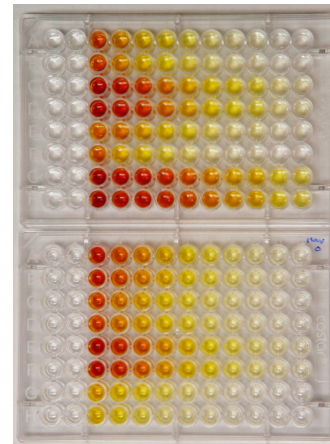
96 well ELISA plates containing duplicate catfish serum samples. Color intensity directly correlates to the concentration of pathogen specific antibody in the serum.
