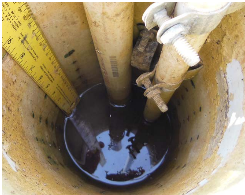
Figure 1. Example of water level measurement below the soil surface using a modified "pani-pipe."
