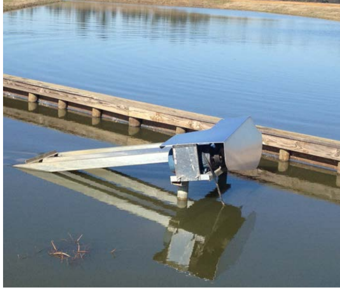
Figure 1. Screw-pump design developed by commercial catfish farmers.
