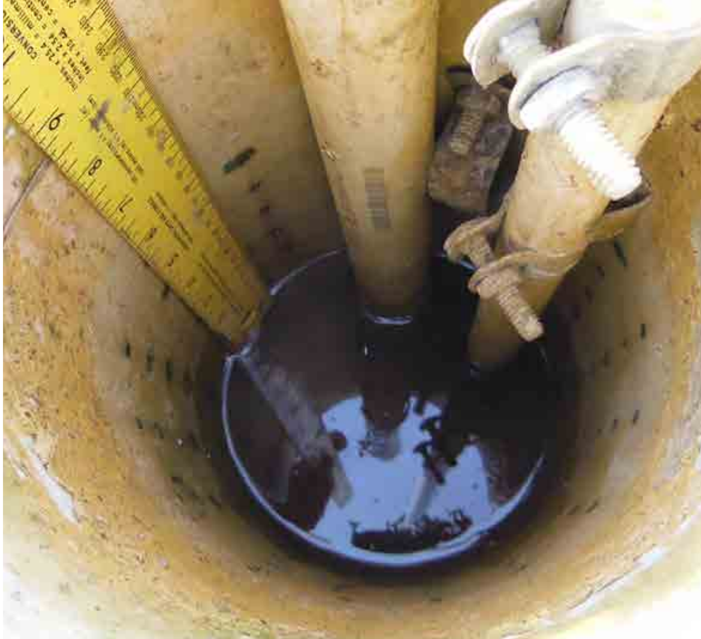
Figure 1. Example of water level measurement below the soil surface using a modified “pani-pipe.”
